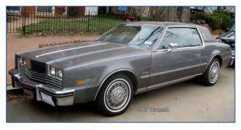
The third generation Toronado (1979–1985) was substantially downsized, losing nearly 1,000 lb and almost 16 inches in length. Reflecting its 206 in length and 114 in wheelbase, it came equipped with the smaller Oldsmobile 350 cu in V8. The engine was rated at 170 HP/270 lb.ft. torque giving it a top speed of over 110 mph and a 0–60 mph acceleration time of 9.4 seconds. This was considered one of the faster times for the "Malaise Era."
